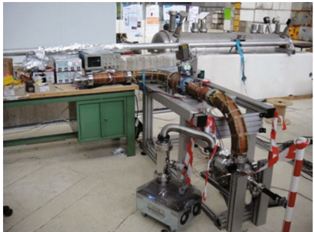
Fig. 2 The slow positron beam line under installation and tests at Saclay
